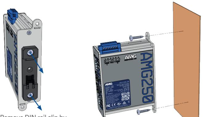
① Remove DIN rail clip by unscrewing the two fixing screws as shown.
