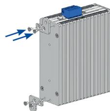
② Attach the wall brackets using the M3x4 fixing screws (included) as shown.
