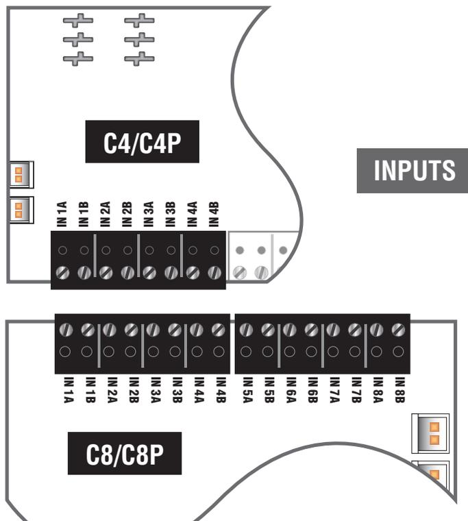
Each input on the **C4/C4P** and **C8/C8P** has an “A” terminal and a “B” terminal.
