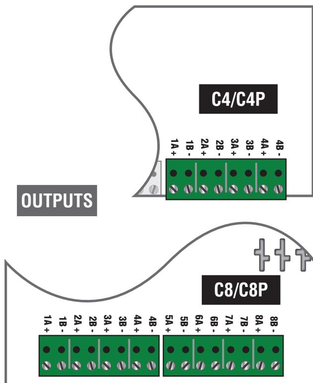
Each output on the **C4/C4P** and **C8/C8P** has an “A” terminal and a “B” terminal. The usage of these terminals varies based on the setting of jumpers **C** and **E** for the zone.
