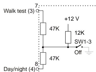
Walk test On = Pin 7 to GND
