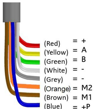
The example below shows how to connect M1 and M2 terminals using the 8x0.22mm unshielded cable.
