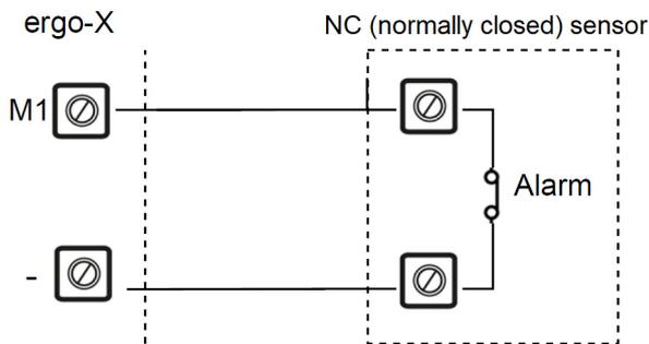
Connect M2 terminal programmed as an output, as the example below:
