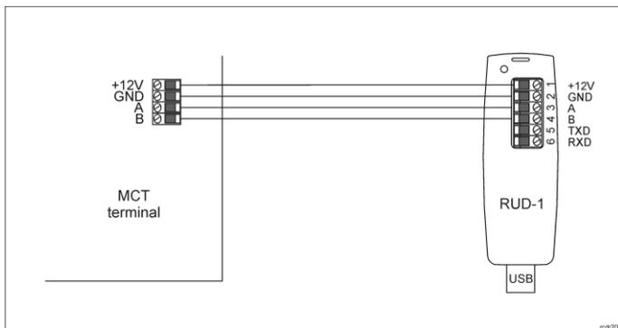
Fig. 1 Connection of MCT terminal to RUD-1 interface
