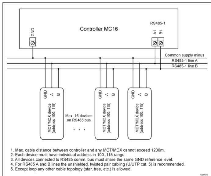
Fig. 3 Connection of terminals and expanders to MC16 access controller
