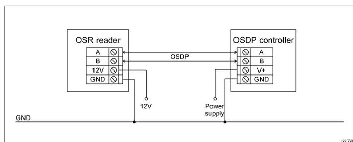
Fig. 3 Typical connection of reader to controller
