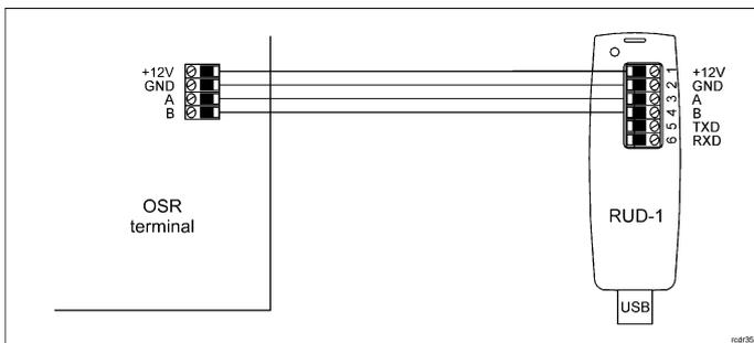
Fig. 1 Connection of OSR terminal to RUD-1 interface
