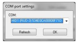
Then RUD-3 must be initialized (Connection > Connect), after this operation device is ready for use.
