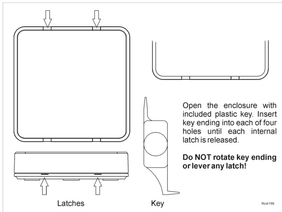
Fig. 9 Front panel disassembly.
