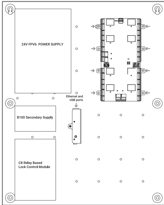
Figure 5 Access Control Core mounted without bracket (Ethernet and USB ports facing up) below 8-Port Board
