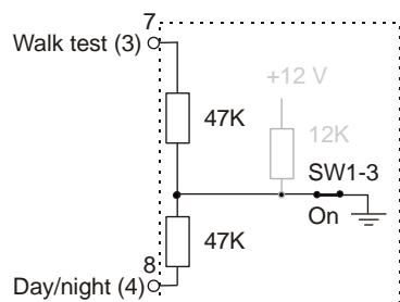
Walk test On = Pin 7 to +12 V
