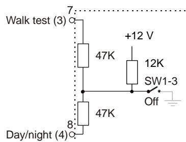
Walk test On = Pin 7 to GND
