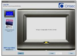
NOTE: If the image being uploaded is bigger than 480x272 pixels the program will resize the image to the required size, the following information box will populate the screen.
