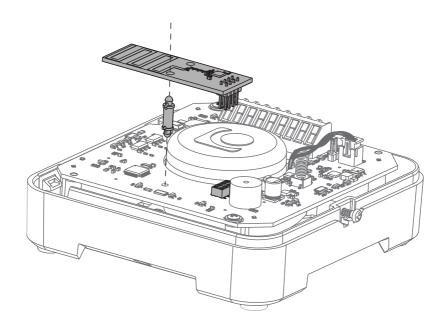
NOTE: Do not add/remove the W-AP whilst the INT-CS is powered.
