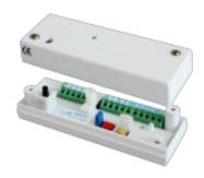
IU 400 is an interface/analyzer for glass break detector GD 475 and shock detector CD 475. It has three relays one for Intrusion, one for Fault and one for Tamper. Max 10 units of GD 475/CD 475 detectors can be connected to one IU 400 unit. IU 400 together with GD 475/CD 475 is certified according to EN 50131-1 and EN 50131-2-7-2:2013 Grade 3, Class II.
