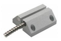
The MC 240-S78 set is intended for exposed environments where a more durable magnetic contact is needed on steel surface or iron doors and gates, etc. The set consists of MC 240-C contact with NC contact function installed in MC 200-7 Al housing and an extra strong magnet in MC 200-8 Al housing, which allows for a wide opening gap.
