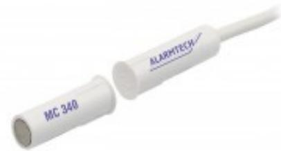
MC 340 is a universal magnetic contact with NC function that can be used in both alarm and access control systems for monitoring e.g. doors and windows against unauthorized opening. Both the contact and the magnet part are encased in a water proof (IP67) plastic housing, which enables easy installation into wood without additional accessories. With our extensive range of installation accessories it is easy to install the contact either recessed or as a surface mount on metal and other materials.
