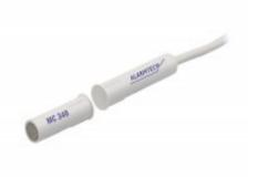
MC 346 is a universal magnetic contact with change-over (NC/NO) function that can be used in both alarm and access control systems for monitoring e.g. doors and windows against unauthorized opening. Both the contact and the magnet part are in a water proof (IP 67) plastic housing, which enables easy installation into wood without additional accessories. With our extensive range of installation accessories it is easy to install the contact either recessed or as a surface mount.
