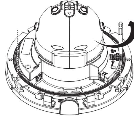
3. Remove the camera body and mounting plate by pulling the mounting clip, as shown in the figure.
