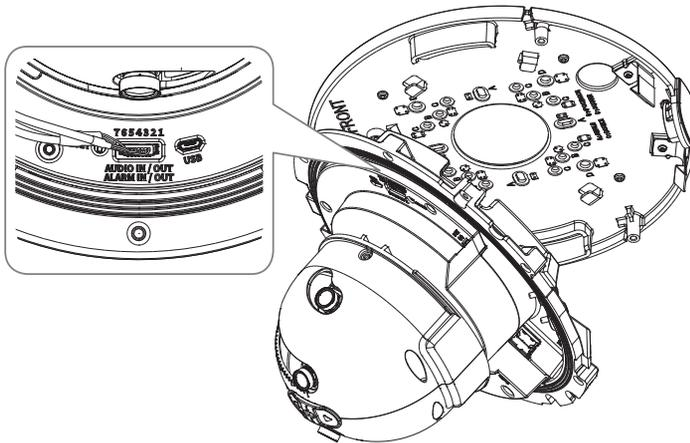
7. Lift up the camera body and push the mounting clips until they click into place.
