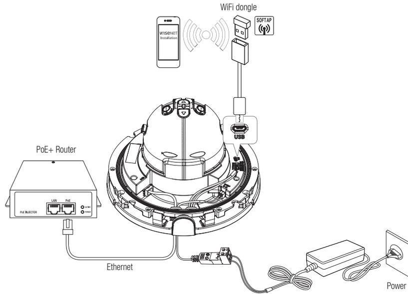
! ■ The Micro USB port of the product is provided for easier installation, and is not recommended for monitoring purposes.
