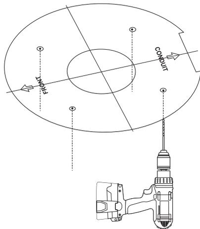
1-2. Fix the mount plate using appropriate screws.
