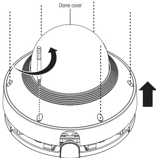
2. Loosen the fastening screw on the camera body.
