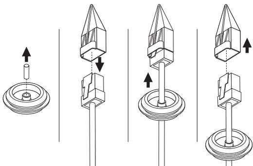
4-4. Connect the network cable jack to the PoE+ port of the camera.
