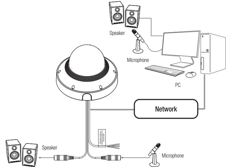
1. Connect the AUDIO IN port of the camera with the microphone or LINE OUT port of the amplifier that the microphone is connected to.
