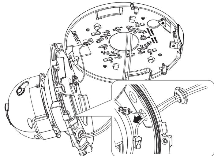
3-5. Connect the network cable connector to the PoE+ port, and connect the power terminal block to the power port.
