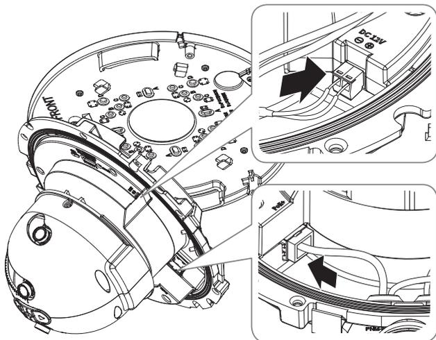
4-3. Mount the cable bushing to the camera body.
