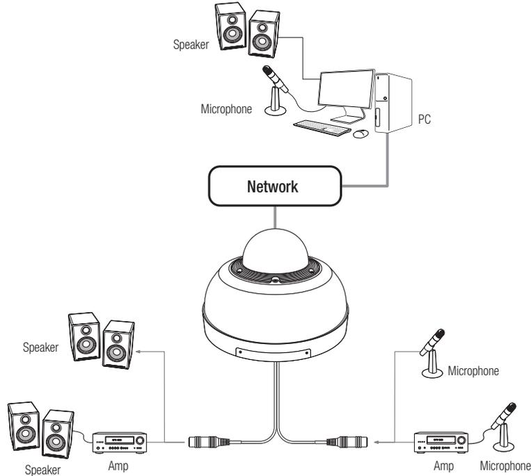
1. Connect the AUDIO IN port of the camera with the microphone or LINE OUT port of the amplifier that the microphone is connected to.
