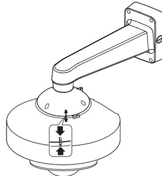
6. Turn the camera in the direction of the arrow so that the installation direction guides at the top and bottom are placed as shown below.
