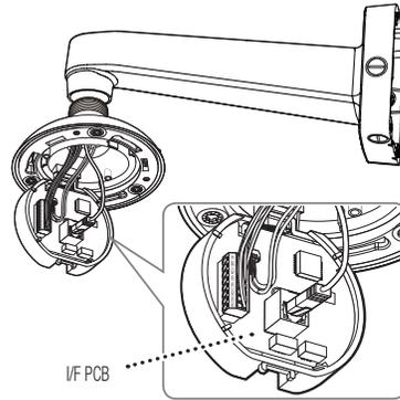
4. After fastening the I/F PCB to the body, install the safety wire of the camera body to the installed base.
