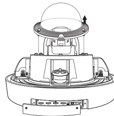
2. Insert a Micro SD card in the arrow direction shown in the figure.
