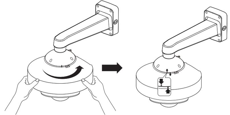
7. Use the screw bit(Torx 30) to secure the installed base and the camera.
