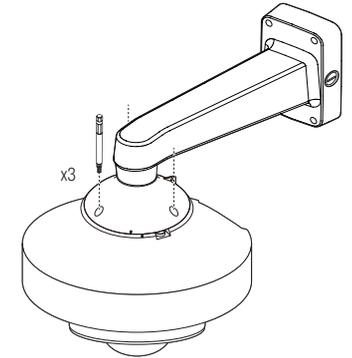
9. Use the Torx L wrench or screw bit(Torx 20) to join the window cover.
