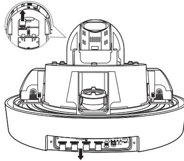
2. Using the Torx L wrench or screw bit(Torx 20), join the dome cover and the micro SD card cover.
