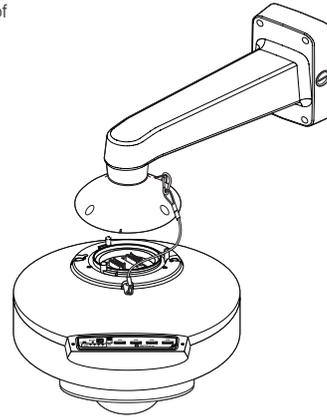
5. Join the installed base and the camera body by matching the Installation direction guides.
