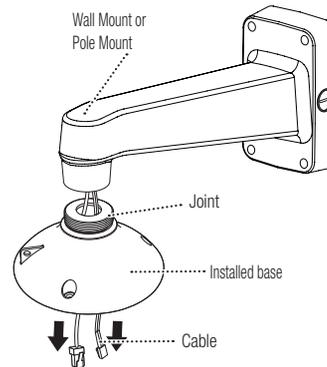
2. Turn the installation base in the direction of the arrow to join it to the mount.
