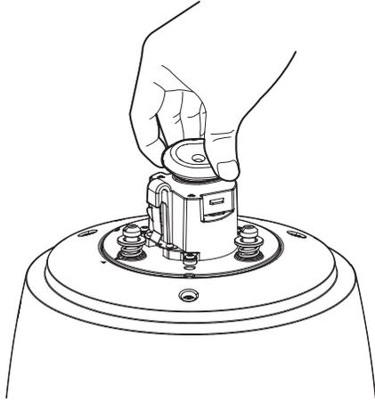
2. Pull off the extruded part of the removed cable bushing.
