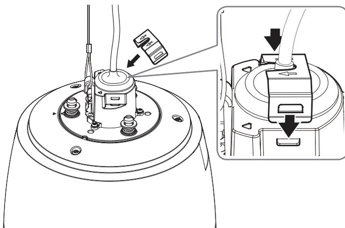
5. After aligning the installation direction guides of the hanging mount, push the main cover upward and turn it counterclockwise until it is secured.
