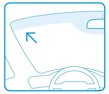
Determine the position of the Booster 2G on the inside of the vehicle's window\*.
