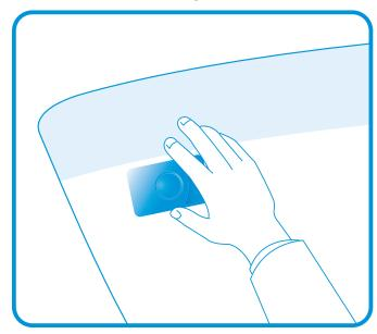
Firmly press the Booster 2G against the inside of the window in line of sight of the TRANSIT reader.
