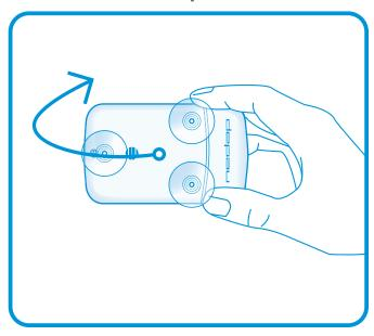
The suction cup is the Booster 2G's front side (active part). This part should face the outside of the window.
