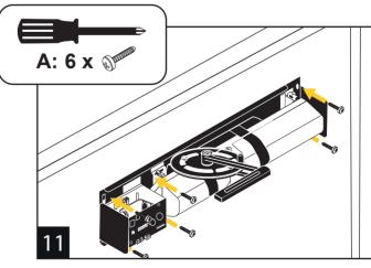
Remove the template from the door and fasten the Freedor into position using the 6 screws in Pack A. Match the orientation of the unit to the template used when making the pilot holes. Ensure the unit is level before tightening the screws fully.
