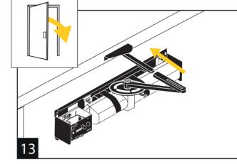
Connect the two halves of the closer arm.
