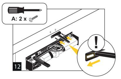
Fasten the other section of the closer arm to the door frame, making sure the base fixing is in the correct orientation, as shown in the template.
