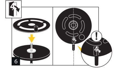
Sit the upper radial disc onto the lower radial disc with the correct number (4) in line with the lower radial disc nib.
