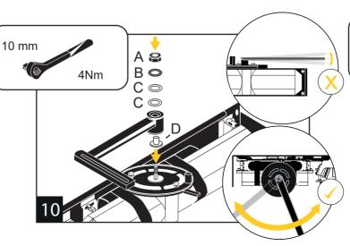
Fit the closer arm to the Freedor unit (closer bolt), ensuring that the washers are fitted in the correct order. Secure the nut using a 10mm socket.
