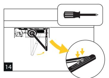
Adjust the arm so that it is perpendicular to the door, then fasten together using the 2 short screws (previously removed in Diagram 9).
