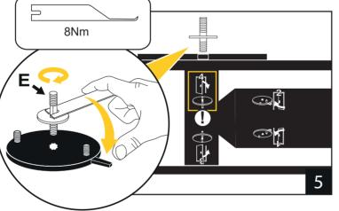
Place the lower radial disc on the square pinion of the closer so that the radial disc nib is facing the same direction as depicted in the graphics.
