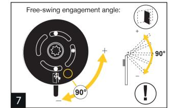
At this point the free-swing engagement angle can be adjusted by rotating the upper radial disc. Keeping the number in line with the nib will give a 90-degree free-swing engagement angle.
