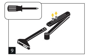
Take the closer arm out of its packaging and disassemble the two parts. Set the short screws to the side for now.
