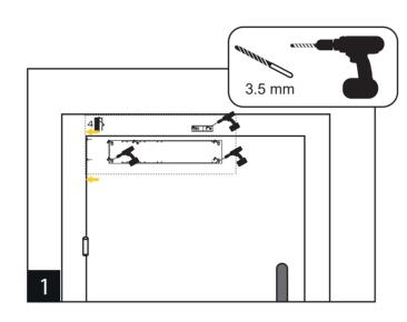
Remove the backing film from the adhesive pads supplied in Pack A and stick on the underside of the Freedor installation template, in the rectangles shown. Remove the top film and align the template with the edge of the hinge side of the door, with the
