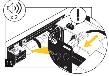
At this stage connect the battery harness cable to the power input connector. The unit will power up, flash its power LED, and beep twice. The Freedor will not engage into free-swing until its cover is on.
