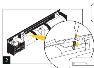
Take the Freedor out of its packaging, remove the 4 thumb screws and slide off the cover. Set to the side for now.
