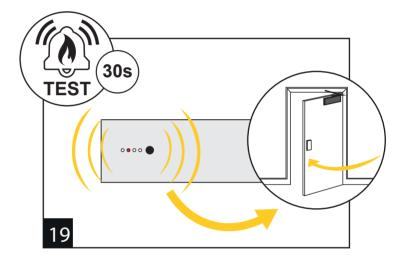
Trigger a fire alarm. The Freedor's FIRE LED will flash RED and the Freedor will release and close the door. Once the alarm test has finished, open the door to engage back into free-swing.
