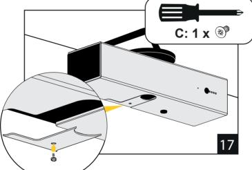
Remove the protective film from the correct blanking plate, and fit to the bottom of the Freedor using the screw supplied in Pack B. Do not fit a plate to the top, as this will prevent the unit from engaging into free-swing.
