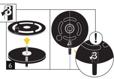
Sit the upper radial disc onto the lower radial disc with the correct number (3) in line with the lower radial disc nib.
