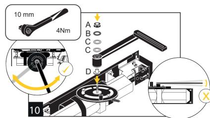
Fit the closer arm to the Freedor unit (closer bolt), ensuring that the washers are fitted in the correct order. Secure the nut using a 10mm socket.
