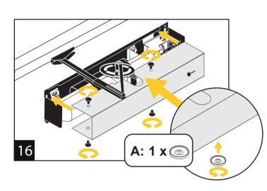
Slide the cover back on, aligning the button with the hole on the front. Fasten in place using the 4 thumb screws.
