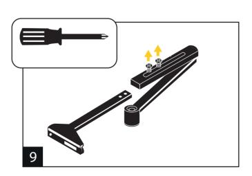
Take the closer arm out of its packaging and disassemble the two parts. Set the short screws to the side for now.
