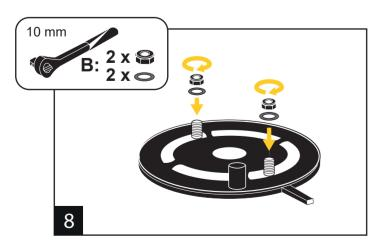
Fasten in place using the nuts and washers in Pack B.
