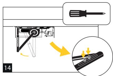
Adjust the arm so that it is perpendicular to the door, then fasten together using the 2 short screws (previously removed in Diagram 9).
