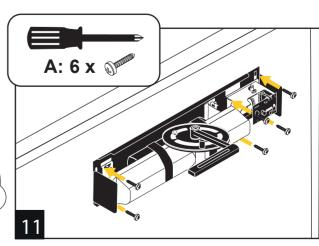
Remove the template from the door and fasten the Freedor into position using the 6 screws in Pack A. Match the orientation of the unit to the template used when making the pilot holes. Ensure the unit is level before tightening the screws fully.
