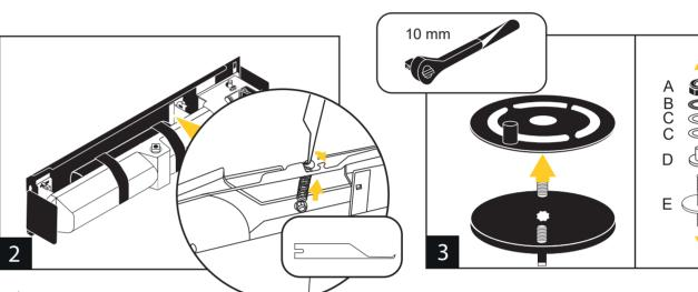
Take the Freedor out of its packaging, remove the 4 thumb screws and slide off the cover. Set to the side for now.
