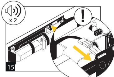
At this stage connect the battery harness cable to the power input connector. The unit will power up, flash its power LED, and beep twice. The Freedor will not engage into free-swing until its cover is on.
