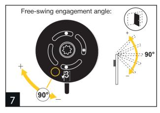
At this point the free-swing engagement angle can be adjusted by rotating the upper radial disc. Keeping the number in line with the nib will give a 90-degree free-swing engagement angle.
