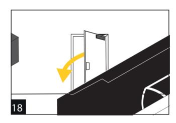
Open the door fully, and the Freedor should engage into free-swing. Leave the door open.
