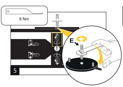
Securely fasten the lower radial disc to the closer with the closer bolt (E) using the other side of the installation tool.
