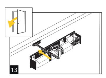
Connect the two halves of the closer arm.
