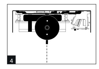
Place the lower radial disc on the square pinion of the closer so that the radial disc nib is facing the same direction as depicted in the graphics.
