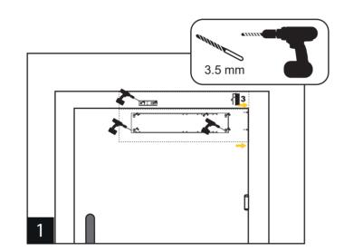
Remove the backing film from the adhesive pads supplied in Pack A and stick on the underside of the Freedor installation template, in the rectangles shown. Remove the top film and align the template with the edge of the hinge side of the door, with the dashed line along the top of the door.
