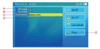
A. IP Address and Mask Display: To change this setting, press the setting key, jump to the IP setting screen, and then change the setting. DHCP and static IP are supported.
