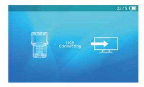
Use a USB mini-B cable to connect the tester to a computer. Further operation is the same as a common USB disk.
