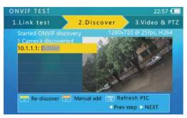
Video information is also displayed above the snapshot, Showing resolution, framerate, and compression method.
