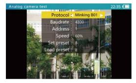
Use the up and down arrow keys to select an item, and the left and right arrow keys to adjust it.
