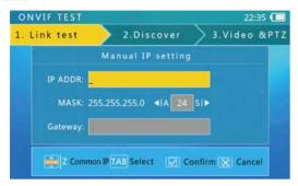
Please use the flip keyboard to input the IP and use the A/S key to adjust the mask. To access internet, gateway access is also needed.
