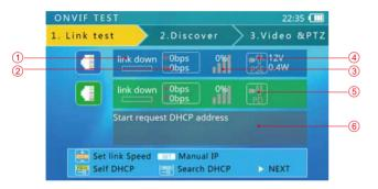
On this interface, blue bar is for network port 1 status information; green bar is for network port 2. The gray bar is IP test information.
