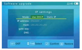
If the network is using DHCP, the tester will automatically detect the IP settings. Otherwise, the IP settings should be entered by the user. Please consult your network manager.
