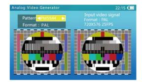
Press the MODE key to select analog video generator. Press the | key or wait 2 seconds to enter the analog video generator function.
