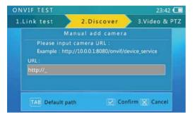
To manually add a camera, the must know the camera's exact IP and ONVIF service path.
