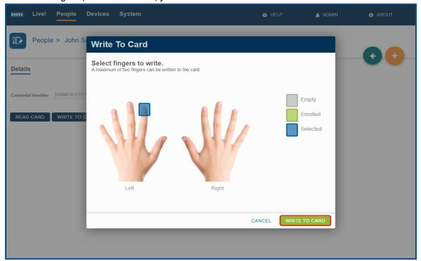
5. You will have approximately five seconds to present the supported card to the Signo Biometric Reader 25B device in order to write the profiles to the card. The LED bar will flash while writing to the card. Keep the card close to the reader until the LED bar returns to it's default color. You will be notified when the card has been successfully written to.
