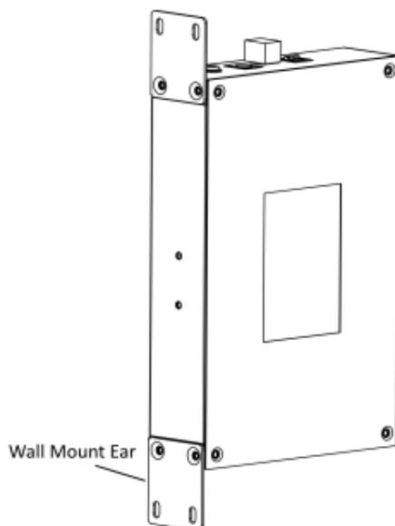
**Figure 2-1 Wall-Mounted Installation**
