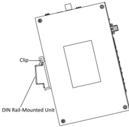
Figure 2-2 Rail Mounted Installation
