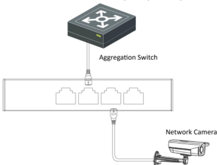
Figure 3-3 RJ45 Port Connection
