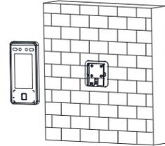
4 Use 1 supplied screw (SC-KM3X6-H2-SUS) to secure the device and the mounting plate.
