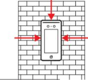
You can also install the device on the wall or other places without the gang box. For details, refer to the User Manual.
