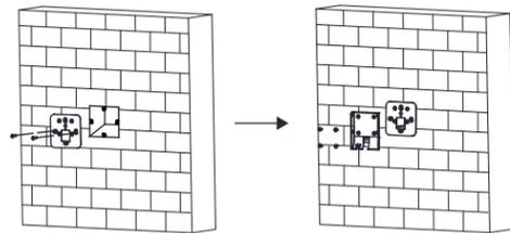
3 Align the device with the mounting plate and hang the terminal on the mounting plate.
