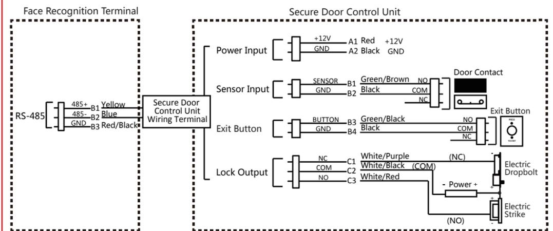
The secure door control unit should connect to an external power supply separately. The suggested external power supply is 12 V, 0.5 A.
