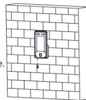
5 Apply Silicone sealant among the joints between the device rear panel and the wall (except the lower side) to keep the raindrop from entering.
