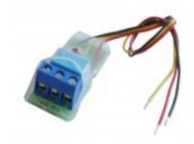
The RC 1 is a very compact and universal relay card with alternating (NC/ NO) relay function. Connection of the relay is provided via screw terminal with wire protection. Control signal and supply is connected via 15 cm cable. Transistor control of the relay means a very low control signal is required (1 mA). An activated relay is indicated via a LED. On the back of the device there is a self-adhesive pad for ease of installation.
