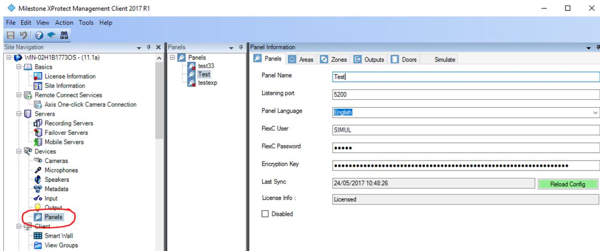
A list of configured SPC Panels is shown. When selecting a panel, the details panes on the right is populated with the configuration of the panel as known in the system.
