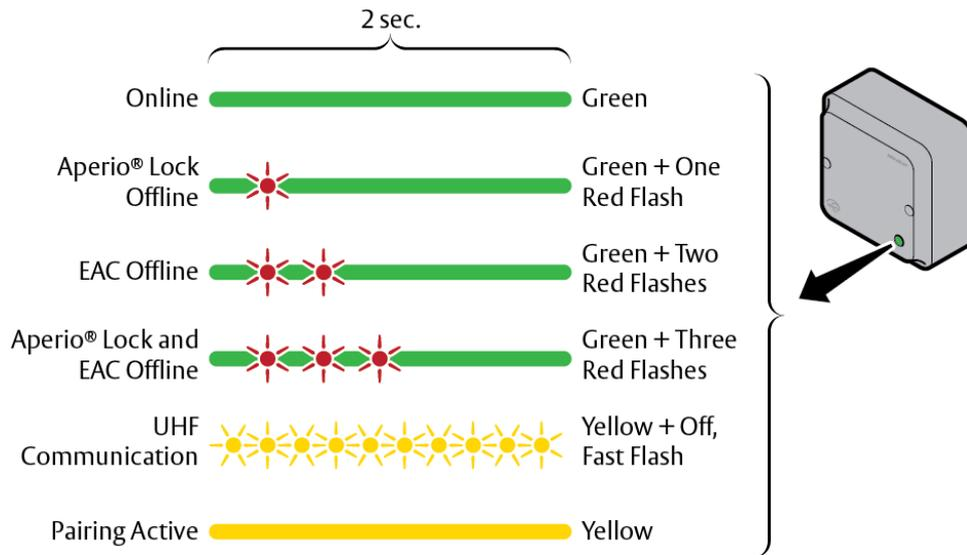
Figur 2. Communication hub normal operation LED indication
