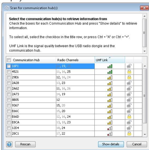
2. Locate a communication hub by the last four characters of the communication hub MAC address (ex. 01CF) in the scan result table. The same characters should be on a label on the cover of the
