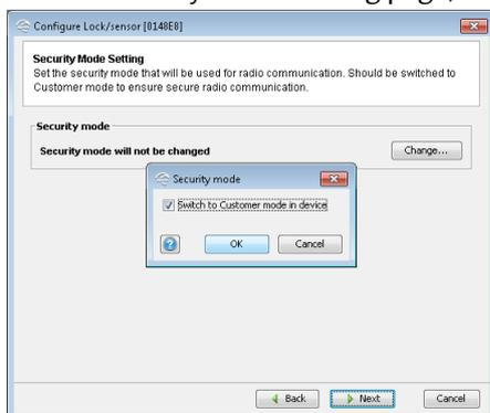
**i** If the installation and first configuration is not performed correctly by setting all locks in customer mode, the radio communication will not be secure and the locks will therefore be vulnerable to intrusion attempts.
