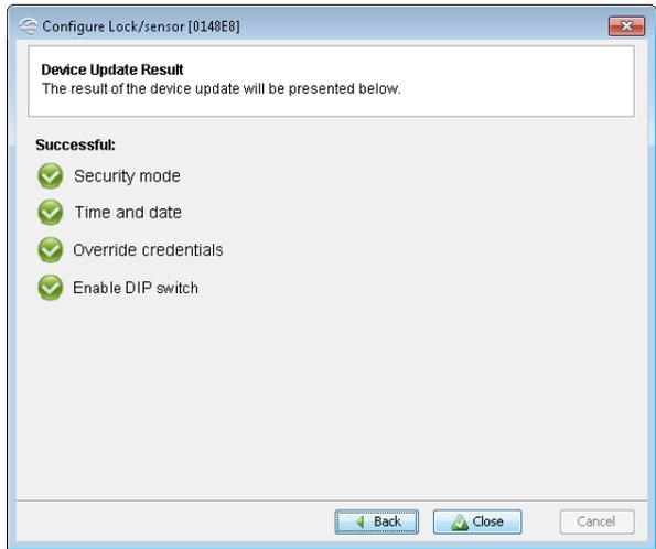
**i** Using the wizard for a communication hub with only one lock paired, customer mode is set both for the lock and communication hub. For communication hubs with several locks paired a security conflict will appear.
