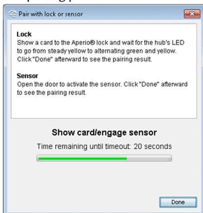
Result: The communication hub pairs with the lock and indicates with one green flash.
