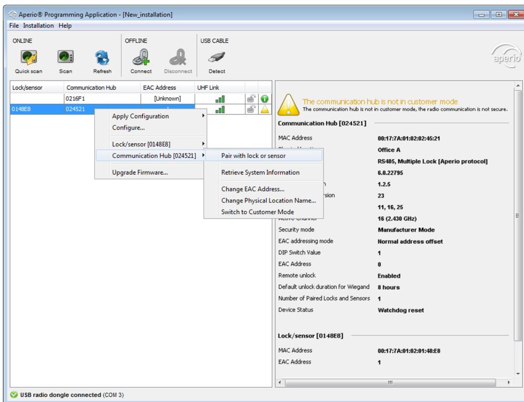
2. The pairing process starts. Hold the credential at the lock, or engage the magnet for the sensor.
