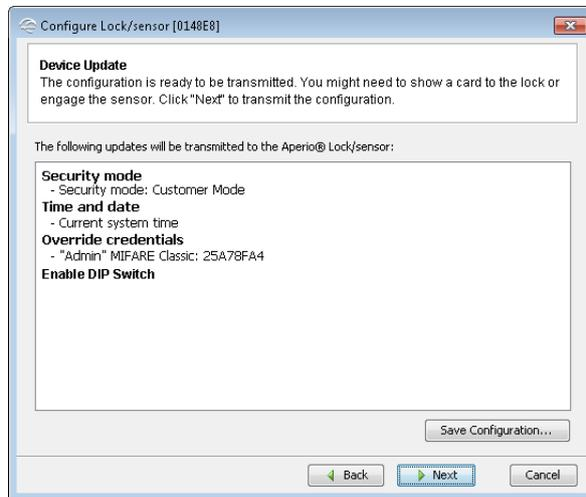
14. If necessary hold the credential in front of the lock to activate the radio.
