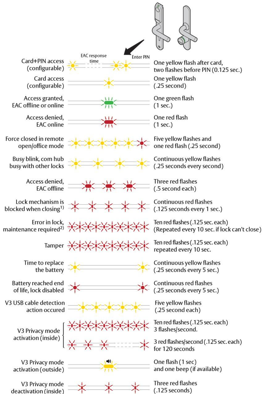
Figure 5: Lock normal operation LED indication
