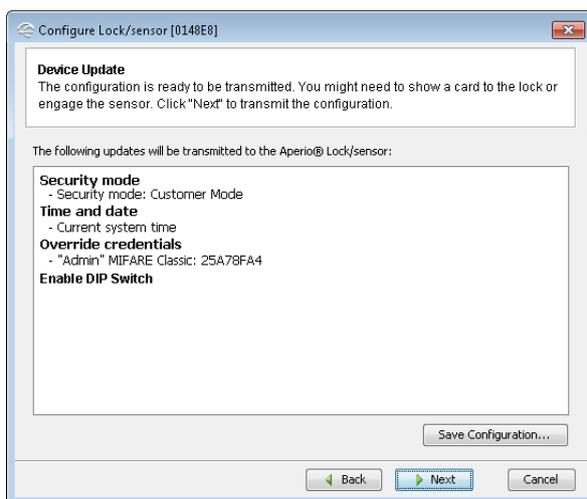
12. Click Save configuration... to facilitate further lock configurations (for other hubs/locks) using the same communication hub. Enter a configuration name and click OK.
