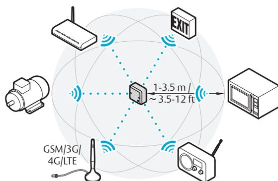
Figure 2. Minimum distance to radio emitting devices
