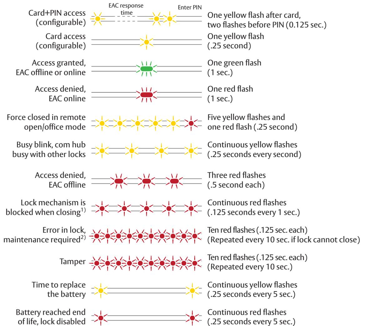
**i** 1) When the lock mechanism is blocked (lock jammed) the knob must be turned/handle released, to release the lock mechanism.
