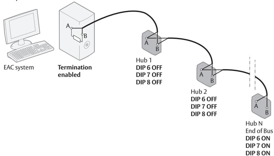
For a star connection, which is not recommended and should only be used in exceptional cases, set DIP 6 and 7 in ON position for one communication hub. DIP 8 must be in ON position for all communication hubs. The RS-485 bus must be terminated on the EAC side as well as on the end hub on each branch.
