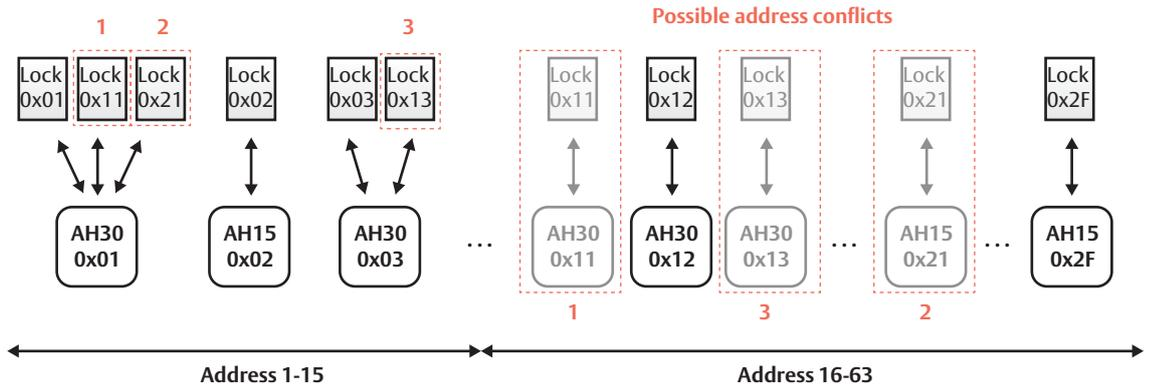
In the address range 1-15, AH30 communication hubs can be used to pair several locks. In the address range 16-63 only AH15 or AH30 communication hubs in single device mode can be used to pair with only one lock. Some
