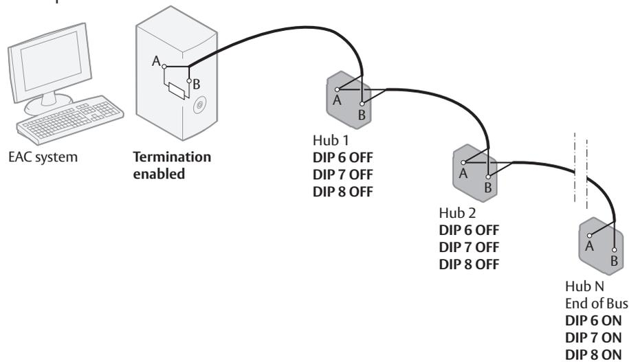
For a star connection, set DIP 6 and 7 in ON position for one communication hub. DIP 8 must be in ON position for all communication hubs. The RS-485 bus can not be terminated on the EAC side.
