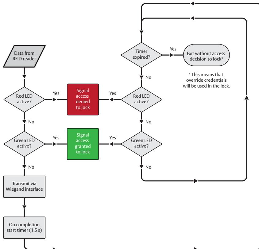
Figure 13. Dip Switch 1 – ON: Access decision logic with two LED signals
