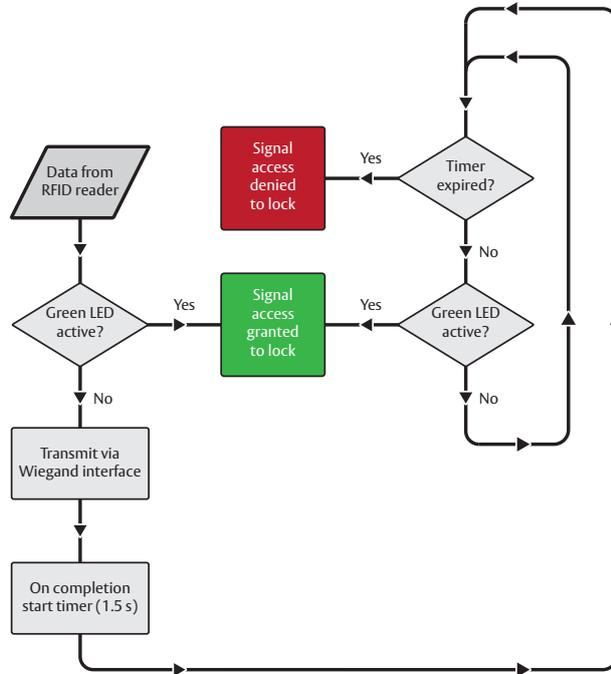
Figure 12. Dip Switch 1 – OFF: Access decision logic with single LED signal
