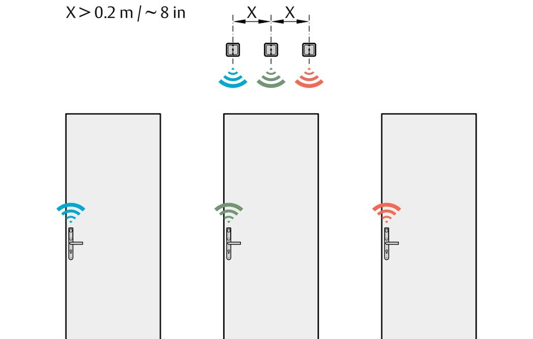
**Placement options for AH15 when using E-cylinder locks**
