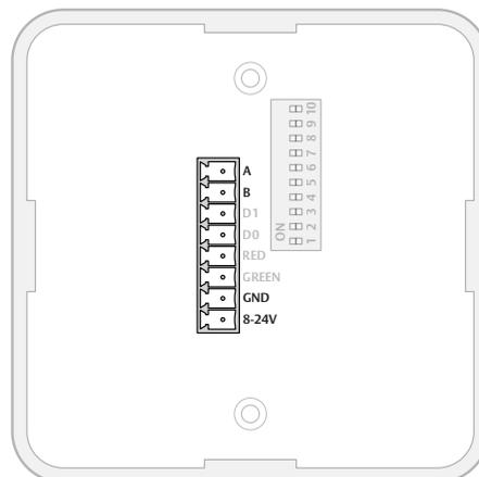
The RS-485 bus should be made up of a twisted-pair cable with characteristic impedance between 90 Ohm and 120 Ohm. Maximum bus length is about 1000 m. Depending on the EAC system, a maximum of 32 units (31 communication hubs plus the EAC, when using the DIP Switch for RS-485-addressing) can be connected to the same bus.
