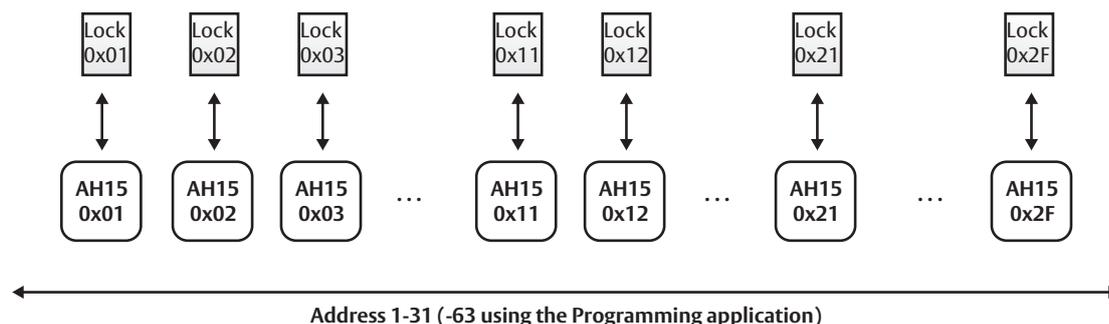
In this installation example, no address conflicts will occur since the lock address is equal to the communication hub address (and provided that the DIP Switches are set correctly with a unique address for each communication hub).
