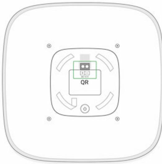
6. Place the front side of the siren on a hard surface and unscrew the 4 screws on the rear panel with a PH2 screwdriver.
