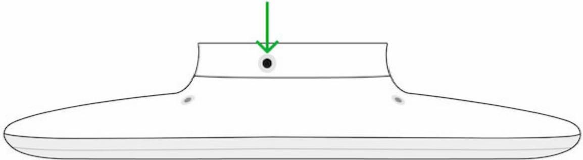
3. Remove the siren from the SmartBracket mounting panel, turning it counterclockwise if the siren is mounted on the mounting plate.
