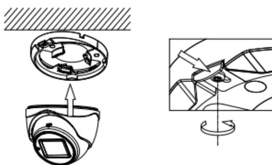
Figure 2-11 Install the Turret Camera
