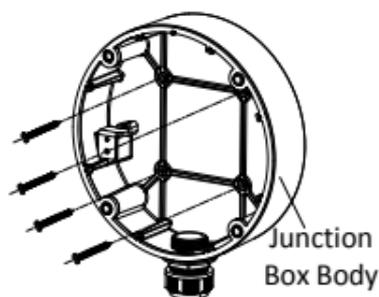
Figure 2-15 Secure the Junction Box's Body on Ceiling
