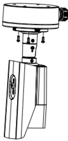
Figure 2-5 Fix the Camera with the Junction Box
