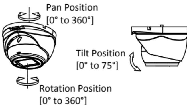
Figure 2-12 3-axis Adjustment
