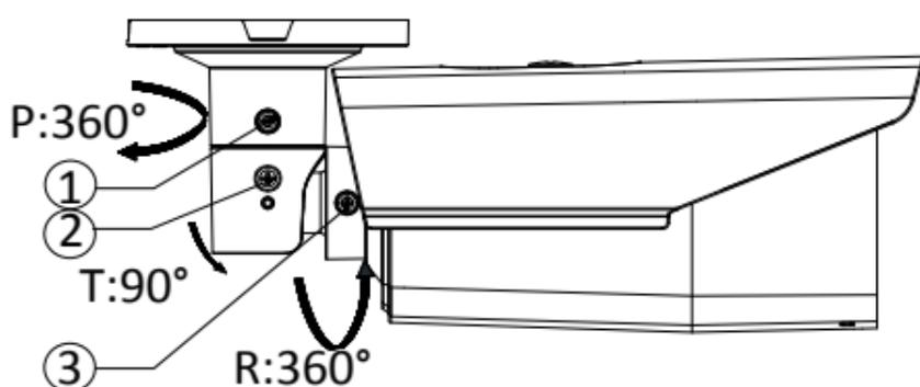
Figure 2-3 3-axis Adjustment
