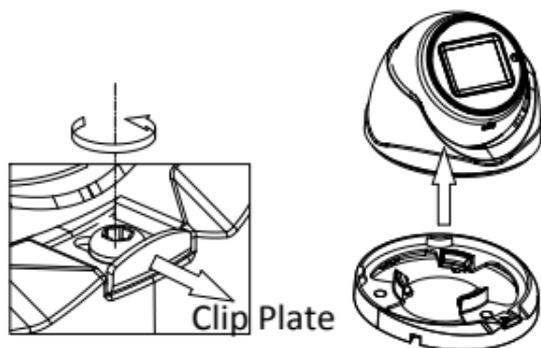
Figure 2-9 Remove the Clip Plate
