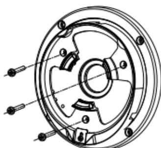
Figure 2-14 Secure Screws on Junction Box's Cover
