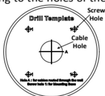
Figure 2-13 Drill Template of the Junction Box
