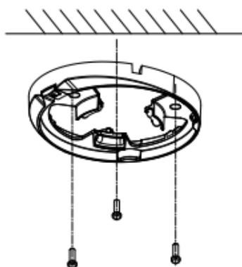
Figure 2-10 Fix the Mounting Base on the Ceiling
