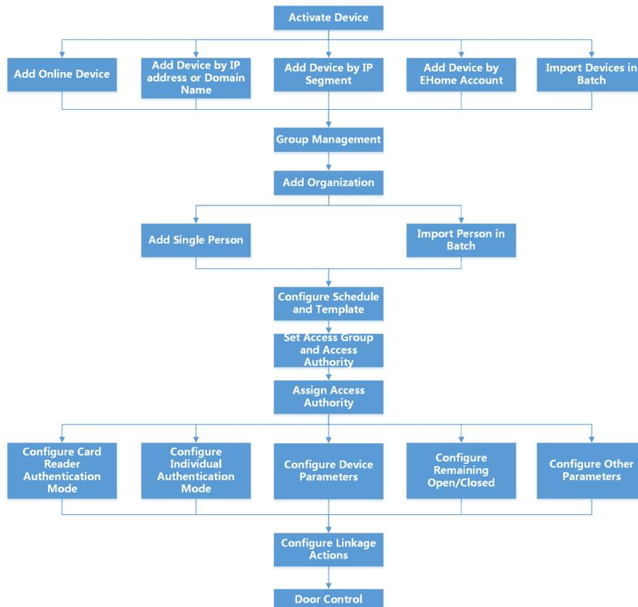
Figure 8-1 Flow Diagram of Configuration on Client Software
