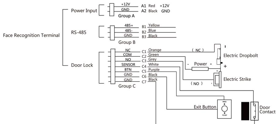
Figure 4-2 Device Wiring
