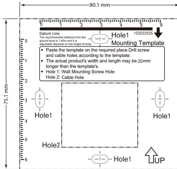
**Figure 3-2 Mounting Template**
