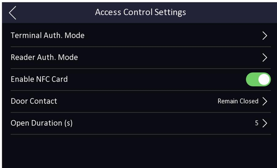
**Figure 6-12 Access Control Parameters**
