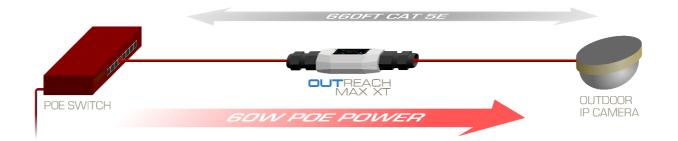
OUTREACH Max XT lets you locate your external IP camera or wireless transmitter right where you want it, without being restricted by the 328 foot limit for Ethernet cables.
