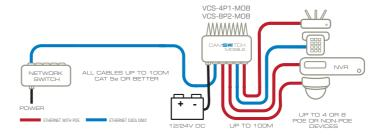
CAMSWITCH 4 Mobile features 4 x 802.3at POE ports, 1 non-POE port, and a versatile DC power input.
