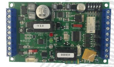
The ViRDI BLC-015 is a single door controller that makes the installation of ViRDI Terminals secure whilst catering to the power requirements of the installations. It utilises ViRDI's RS-485 Secure Transmission Protocol but also can accommodate 3rd Party Wiegand 34bit devices. It has the capability to charge a 12V back-up battery by increasing the voltage from 12V to 13.8V and has drop-out protection. The ViRDI ACC150 switch-mode power supply is utilised with the BLC-015
