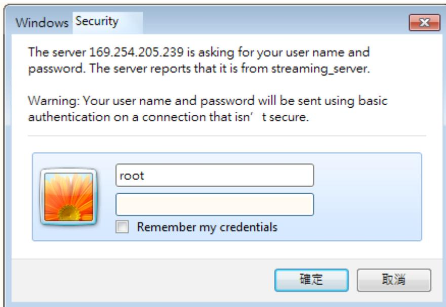
8-2. Enter the combination of alphabetic and numeric characters to fulfill the password strength requirement. The default name for the camera administrator is “root”, and can not be changed.
