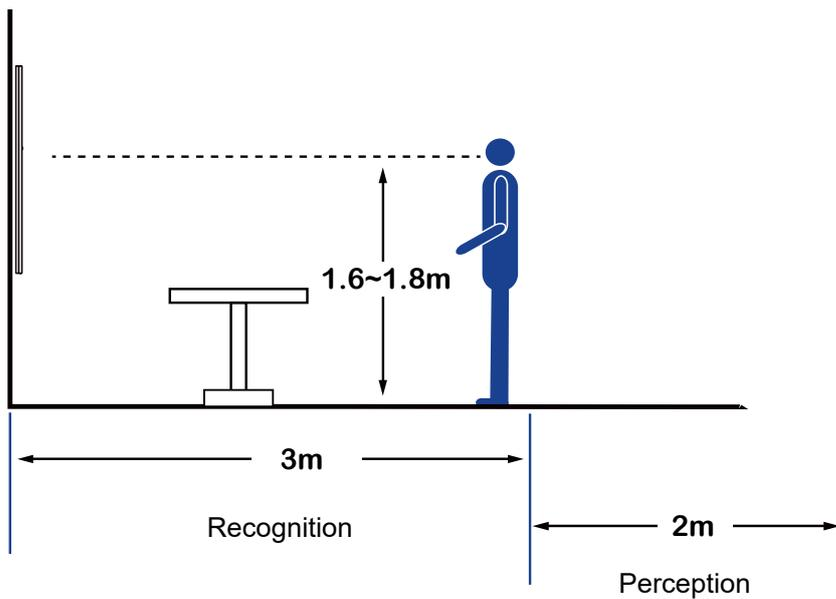
The camera is designed to capture human activities in a near-hemispheric field of view, at a place such as the entrance to a business facility. Due to the optical characteristics of wide-angle lens, image quality decreases as distance from an object increases. It is therefore recommended to install the camera within 3 meters or closer to the objects of your interest. The focus center should also be aligned with objects of importance, say, human faces.
