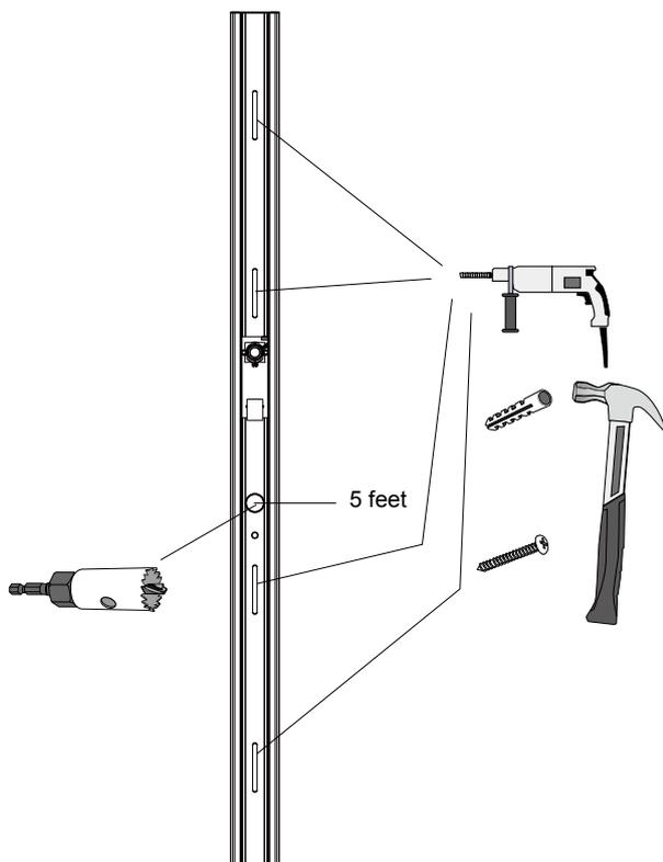
6. When the camera is mounted to wall, connect a CAT5e Ethernet cable to its LAN port, and pass the other end through the routing hole.
