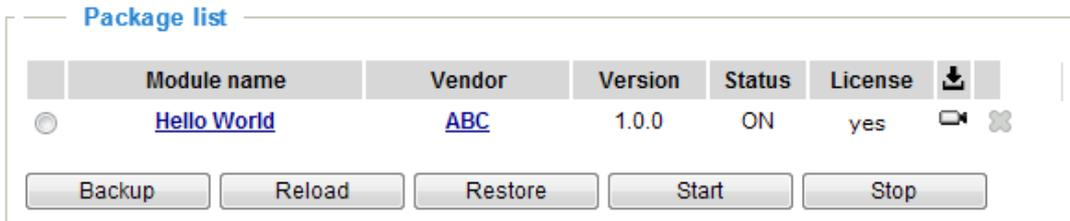
If you should need to remove a module, select the checkcircle in front and then click the **Stop** button. By then the module status will become **OFF**, and the **X** button will appear at the end of the row. Click on the **X** button to remove an existing module.
