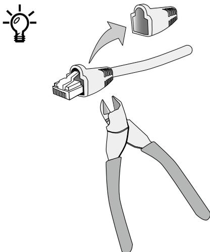
It is recommended to use an Ethernet cable without the connector jacket.
