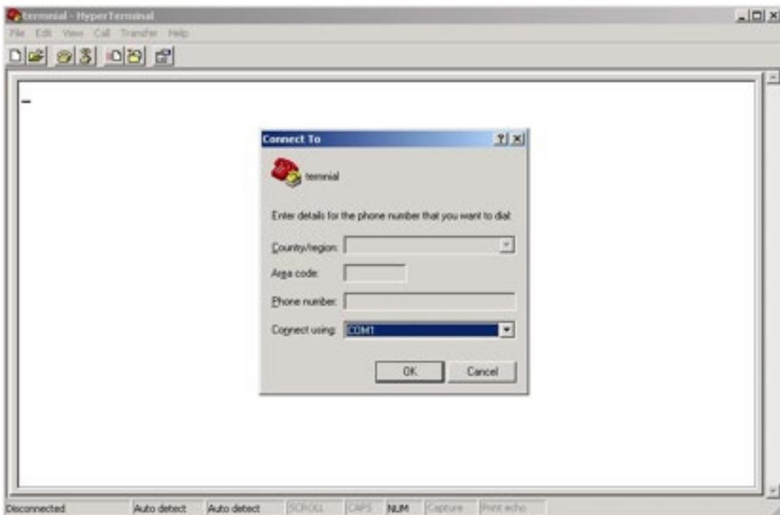
Step 4. The COM port properties setting, 115200 for Bits per second, 8 for Data bits, None for Parity, 1 for Stop bits and none for Flow control.
