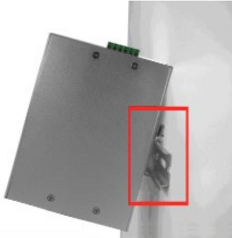
Step 2: Push the switch toward the DIN-Rail until you hear the spring snap into place
