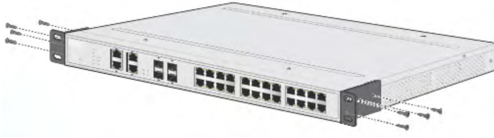
Figure 2-1. Installing the Rack Mount Brackets
