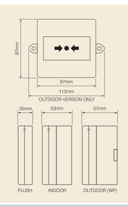
The CXM provides simple changeover contacts for use with a wide range of fire systems or in other applications requiring switching at up to mains voltage.
