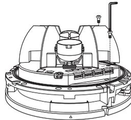
3. Remove the camera body and mounting plate by pulling the mounting clip, as shown in the figure.
