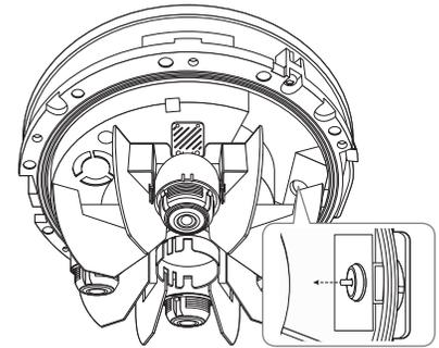
4. Use the Cap Installer to allow the RJ45 cable to pass through.
