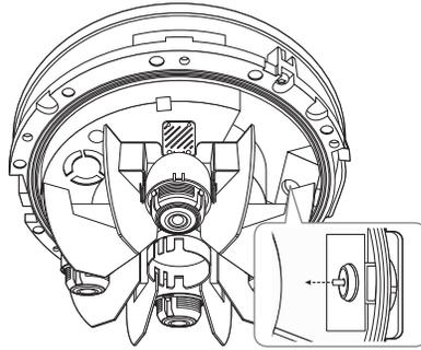
3. Insert the LAN cable through the hole appeared after removing the projected part in step 2 above.
