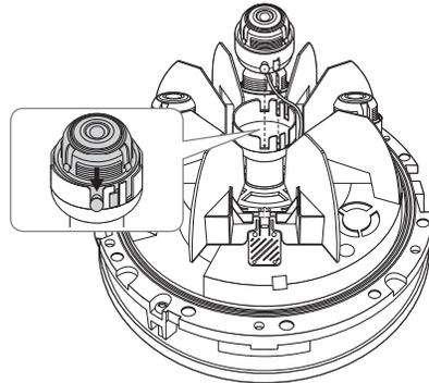
3. Lift the part with diagonal lines to release the frame wall.
