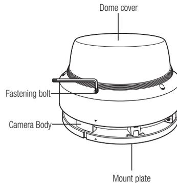
2. Loosen the fastening screw on the camera body.
