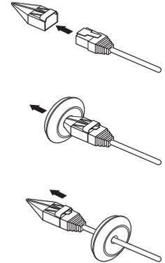
5. Insert the rubber stopper again and connect the LAN cable to the Ethernet terminal.
