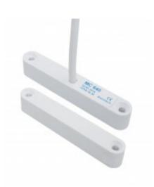
MC 640 is a magnetic contact with NC function that can be used in both alarm and access control systems for monitoring e.g. doors and windows against unauthorized opening. Both the contact and the magnet part are in a water proof (IP 67) plastic housing for recessed and surface installation. The accessory MC 600-1 is a flange for installation in hollow profiles or window frames.
