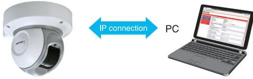
PoE enabled Redscan mini generates Redwall Event Codes (REC) to all compatible VMS and NVR., through a single cable.
