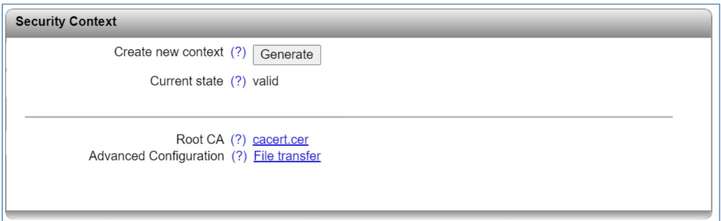
**Create new context:** Clicking on the “Generate” button creates all the necessary keys and certificates for operation with HTTPS and SSH.
