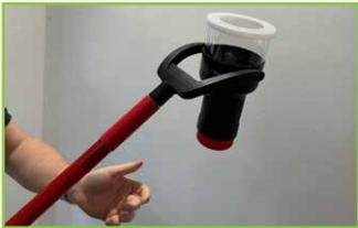
5. Make sure the Head is fitted into the pole securely.
