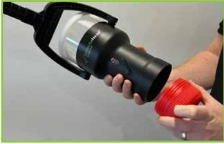
1. Unscrew and remove the retainer cup.
