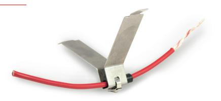
Beam clips may be used to support linear heat detection cable directly (in this case a separate silicone sleeve is required) or fixed to other mounting brackets and used to affix the bracket to a RSJ/I-beam or equivalent.
