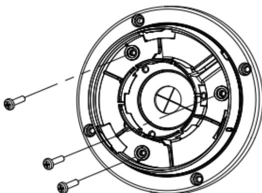
Figure 2-6 Secure screws on the Junction Box's Cover
