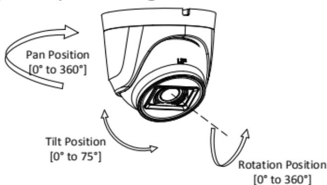
Figure 2-12 3-Axis Adjustment
