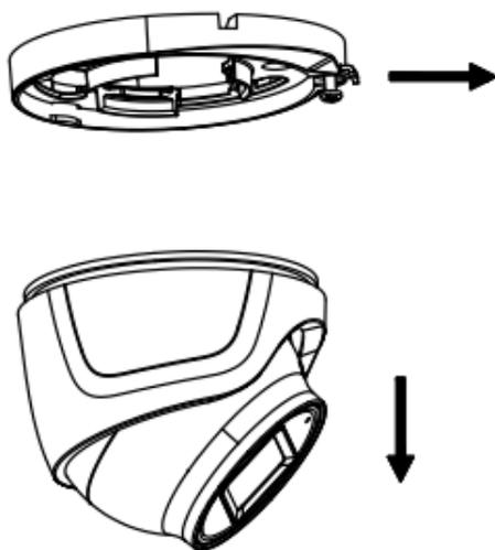
Figure 2-17 Remove the Mounting Base
