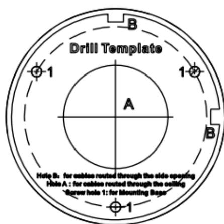
Figure 2-13 Drill Template of the Junction Box
