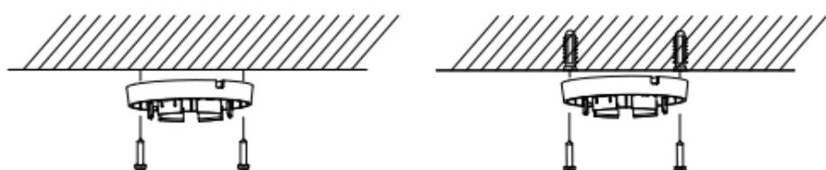
Figure 2-10 Attach the Mounting Base to the Ceiling
