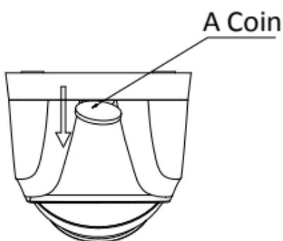
Figure 2-9 Pry the Mounting Base
