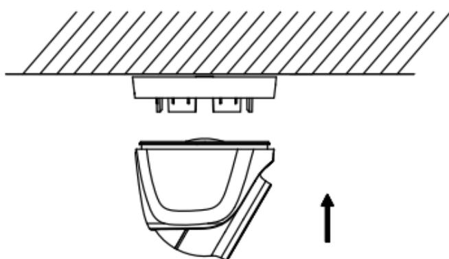
Figure 2-11 Install the Camera Back
