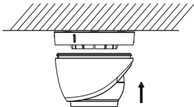
Figure 2-4 Install the Camera Back
