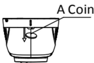
Figure 2-2 Pry the Mounting Base
