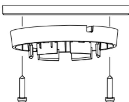
Figure 2-14 Install the Mounting Base
