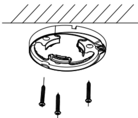
Figure 2-18 Secure the Mounting Base to the Ceiling
