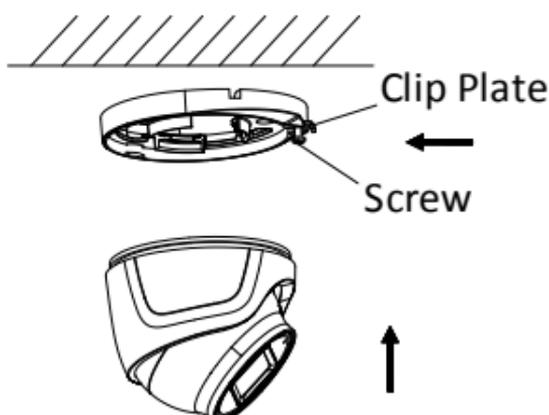
Figure 2-19 Secure the Camera
