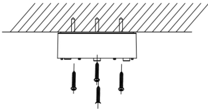
Figure 2-15 Secure the Junction Box on the Ceiling
