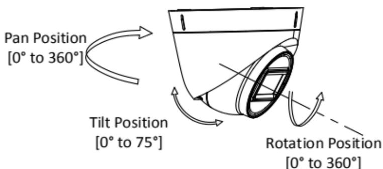
Figure 2-5 3-Axis Adjustment
