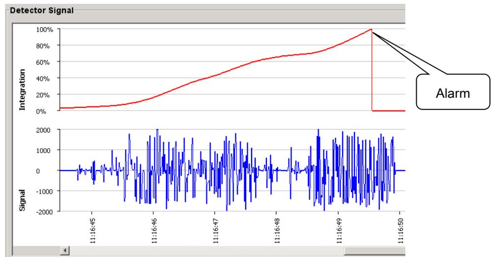
The detector signal recording is shown in blue in the bottom section of the screen. The time stamp is linked to the PC's clock and is implemented when the recording starts. The signal strength automatically adjusts to the strength of the signal being detected, in a range of 0 to +/- 2000.
